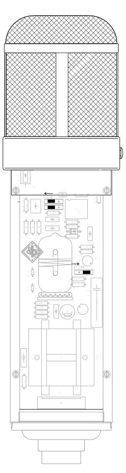
Pure Tube Mode: Jumper shown in Pure Tube Mode Position
