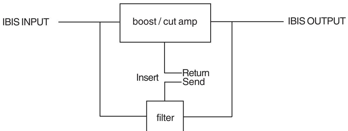
There are 4 filter circuits in parallel in Ibis. When using the insert with a compressor you are modifying the filter output before it sums back into the audio path. The inserts are unbalanced
