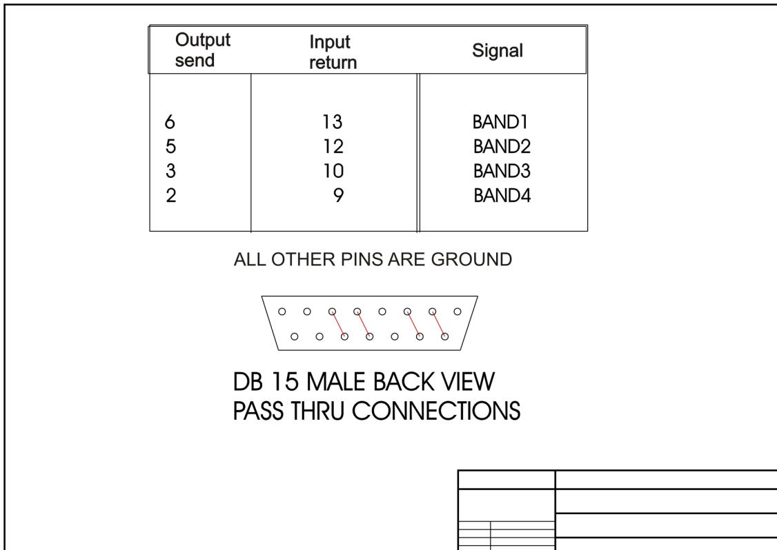
If you are going to use this, use it with caution. The inserts are a loop and must be normaled for the band to work correctly. If there is a phase inversion in the inserted device it is possible that the system will be an oscillator. This will not hurt Ibis, but your Speakers.
