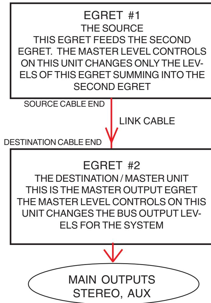
In this configuration each of the two Egrets has 8 digital / analog inputs for a total of 16 inputs. Linking the units together works by tying the summing bus inputs to the appropriate outputs. The source and destination units are selected by how the link cable is plugged in.
