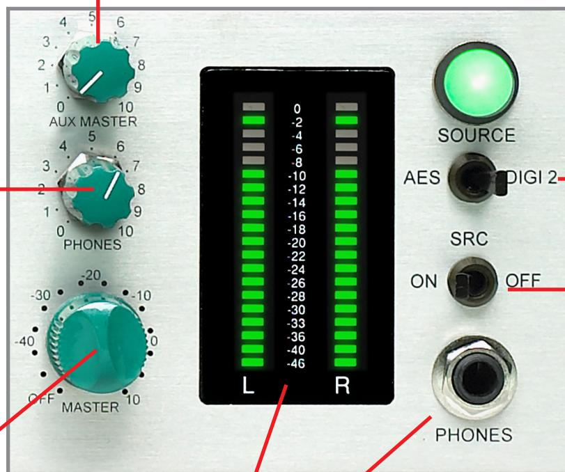
**MASTER** THIS IS THE STEREO BUS LEVEL. AND IS A STEPPED ATTENUATOR. THE GREEN LED SHOWES THE LEVEL SETTING
