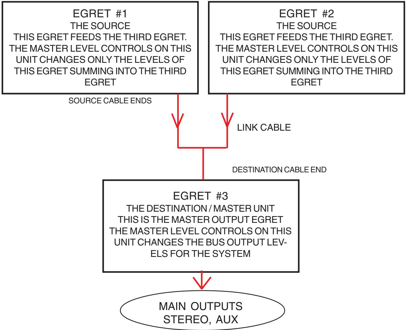
In this configuration each of the three Egrets has 8 digital / analog inputs for a total of 24 inputs. Linking the units together works by tying the summing bus inputs to the appropriate outputs.
