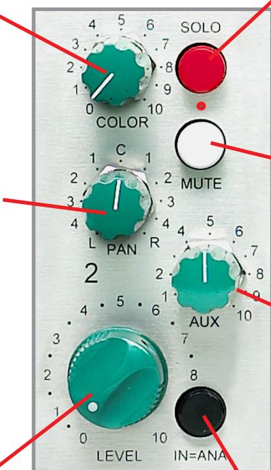
**SOLO BUTTON** BY PRESSING THIS IN THE CHANNEL IS SOLOED THE RED LED LIGHTS ON ALL MUTED CHANNELS
