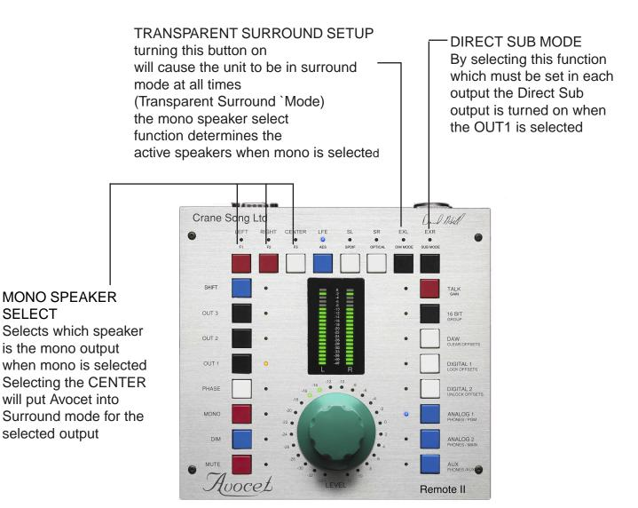
The OUTPUT LEVEL of each speaker may be trimmed down for speaker level matching. When setting up the system so that the normal listening level is around 0 on the dial. When entering the speaker / output setup. No reduction in level is indicated with the level leds showing 0. The speaker trims are in 0.25 db for a max trim of -15.75db. There are 4 steps per db or 8 steps to get to the -2 setting on the dial.
