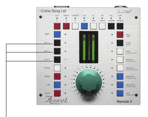
By pressing any one of the speaker select buttons a second time and holding it for about 0.5 seconds will put Avocet into the speaker set up mode.
