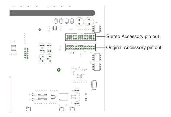
Avocet IIA shipped configured for stereo will have the Accessory connector configured in the stereo mode. This uses the Tascam style of signal assignment. Any one who upgrades from and earlier version and uses the Accessory connector may need to move the internal ribbon cable
