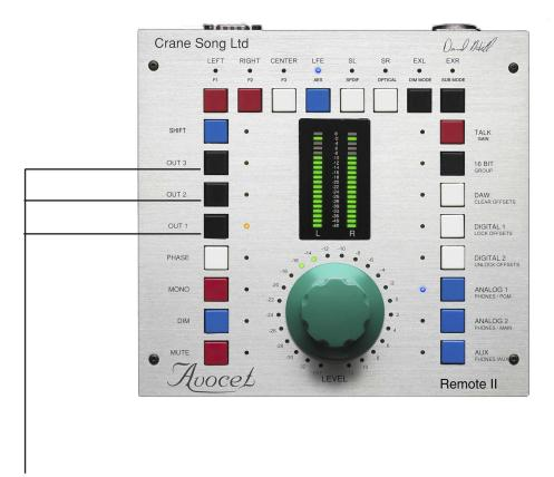
By pressing all three output selection buttons at the same time Avocet will reset all of it's internal settings. This is the same as rebooting the remote.
