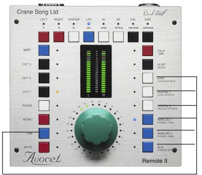
Gain Trims are adjustable by plus or minus 10db on all INPUTS and the MONO function in surround
