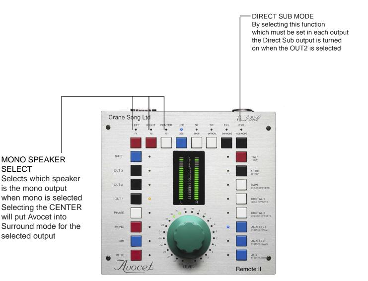
The OUTPUT LEVEL of each speaker may be trimmed down for speaker level matching And setting up the system so that the normal listening level is around 0 on the dial. When entering the speaker / output setup. No reduction in level is indicated with the level leds showing 0. The speaker trims are in 0.25 db for a max trim of -15.75db. There are 4 steps per db or 8 steps to get to the -2 setting on the dial.
