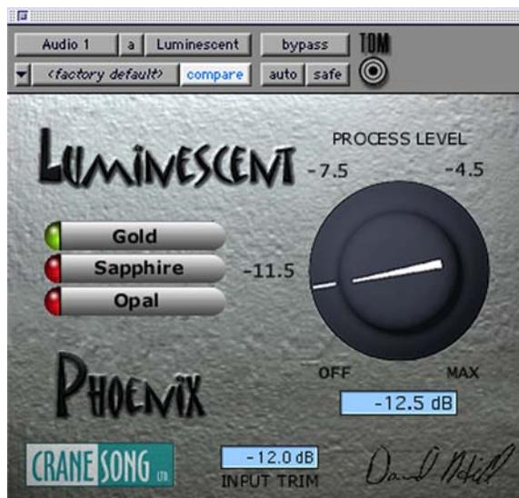
By grabbing the text "INPUT TRIM" with the mouse and moving in the vertical direction the input trim level can be adjusted. It can also have a value between 0 and -12db entered into the window. The Process level can be moved by a mouse by grabbing it's knob and moving the mouse vertically. It can also have a value entered into it's window with 0 db being the maximum value. Phoenix is mono, multi-mono, stereo and 5.1 capable.
